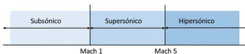
Figure 2. Speed ranges according to Mach number.
